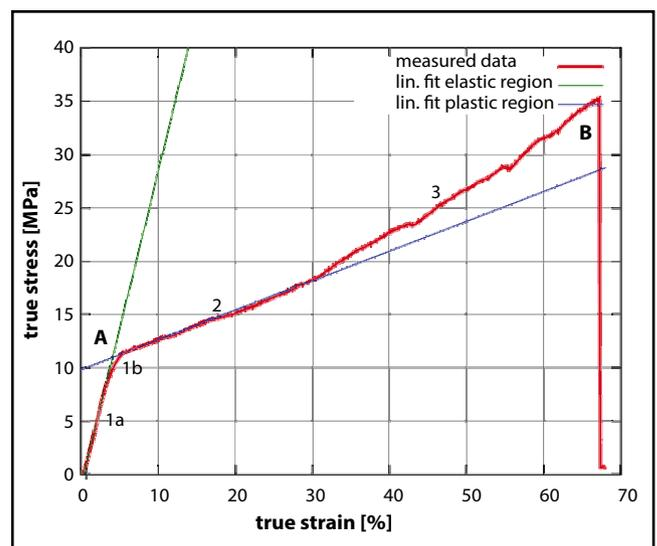
Fig. 5. Load curve obtained from the tensile test of a hair
