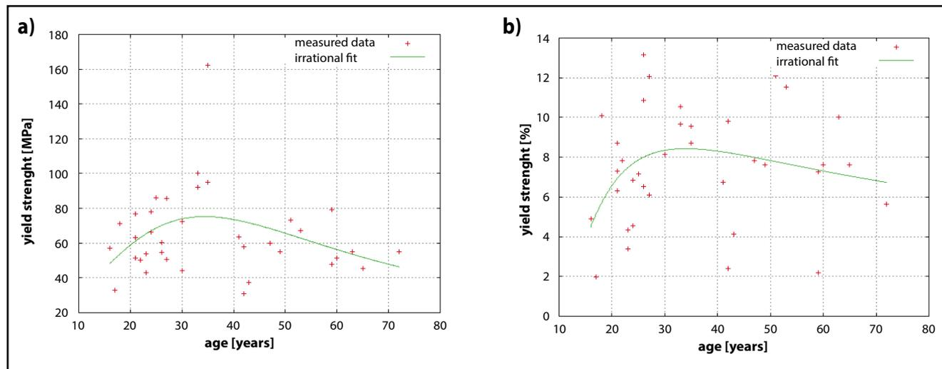
**Fig. 7. a)** Dependence of yield strength [MPa] on a woman's age – approximation by a rational function. The coefficients of approximation equation No.1 are in Table 1. **b)** Dependence of yield strength (in percentage of elongation of hair) on a woman's age – approximation by a rational function. The coefficients of approximation equation No. 1 are in Table 1.
