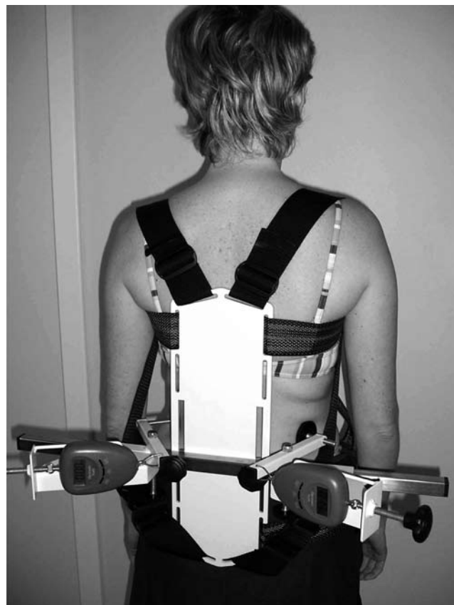
Figure 1. Illustration of strapping of the muscle dynamometer onto an examined subject
